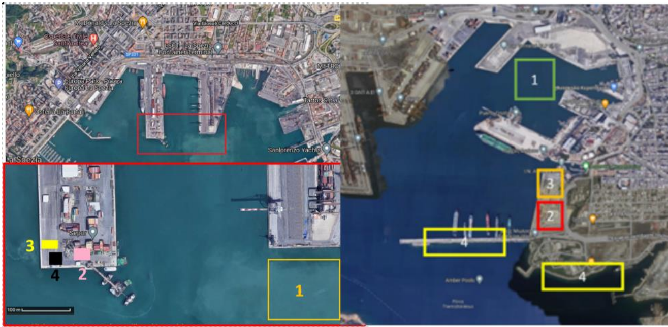
Fig. 2.5.2 - Replication 1. La Spezia port (AdSPMLOr). Key: (1) area for sediment dredging and sampling; (2) area for sediment storage in tanks; sites where installing (3) paving blocks and (4) physical models.
