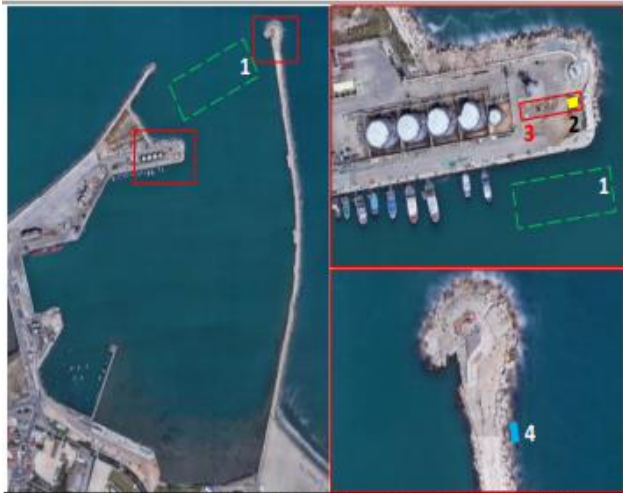
Fig. 1.4.4 - Map of Barletta port (AdSPMAM) showing the sites for the realisation of real-scale products. Key: 1) possible site for sediment dredging and sampling; 2) sediment storage in tanks; 3) laying outdoor paving blocks; 4) installing breakwater revetment blocks.
