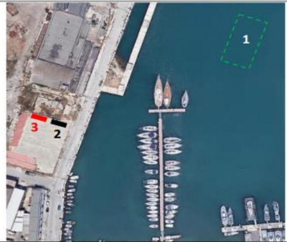
Fig. 1.4.5 - Map of Bari port (AdSPMAM) showing the sites for the realisation of real-scale products. Key: 1) site for sediment dredging and sampling; 2) sediment storage in tanks; 3) installing physical models.
